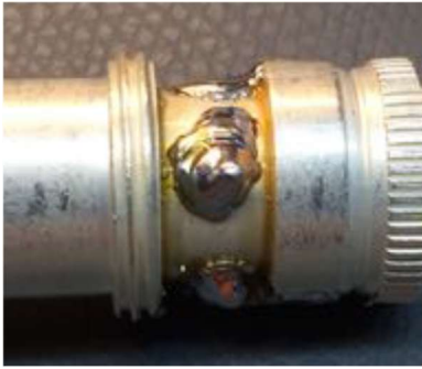
"Bad Solder Job!"
